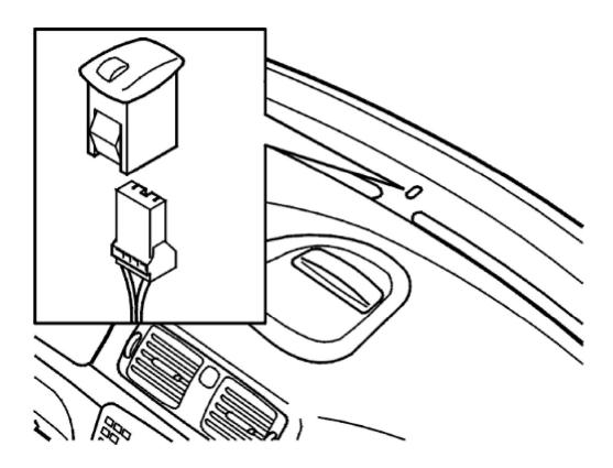
Lift the dashboard over the gear selector lever.
