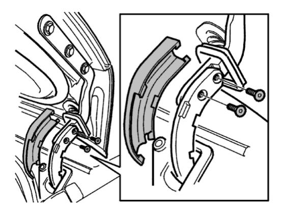
The hinge on the tailgate can be separated in the center. This means that the tailgate does not need to be aligned.
