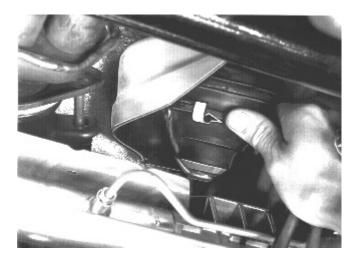
Remove the engine pad by lifting the collision protection system and engine mounting slightly.
