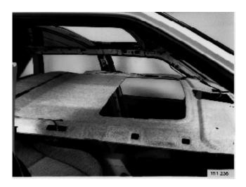
Carefully place headlining over front seal folded backrests and dashboard
