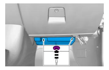
Remove glove compartment Refer to: Glove compartment.
