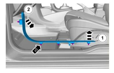
Remove control module relay box passenger compartment Refer to: Control module relay box passenger compartment.
