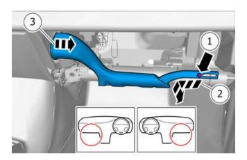
Remove instrument panel lower Refer to: <u>Instrument panel lower</u>,
