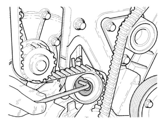
Slacken off the center screw for the belt tensioner slightly.
