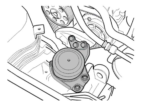
Screw the engine mounting into place on the engine. Tighten to 67 Nm .
