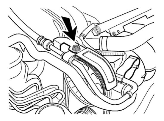
Remove the metal bracket for the servo hose from the rotation protection for the auxiliaries belt.
