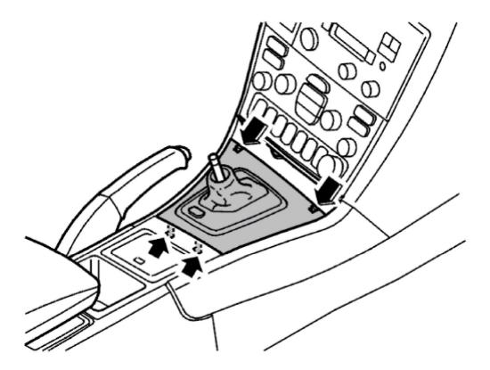
Press in the catches. Angle up the panel at the front edge. Lift the panel out of the rear mountings.
