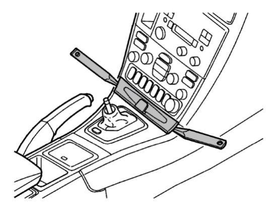
Remove the panel (the pen holder) between the dashboard center console and the center console. Pry out the panel at both ends. Use a weatherstrip tool. Pull the panel straight out.
