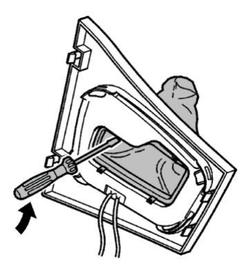
Press out the 4 catches from the top panel. Remove the boot.
