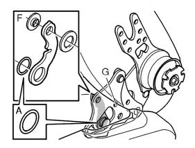
Remove the whiplash element by twisting it and angling it out.
