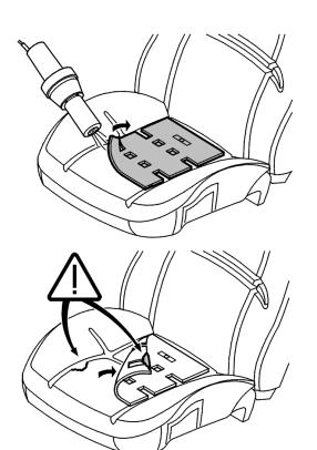
Note! Ensure that the foam filling is not damaged when removing the heater pad. Ensure that the pad is detached from the foam filling. This is to prevent functionality problems when the new heater pad is installed.
