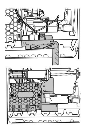
Remove the plastic clip around the electric motor.
