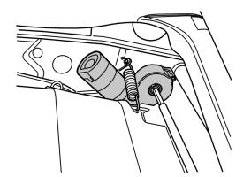
**Hint:** Note the routing of the wiring to make it easier to reinstall.
