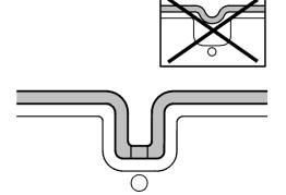
If the heater pad is the type where the pad and/or cable is placed in the channel, the pad must follow the foam filling as illustrated. If not, the pad and/or cable may be loaded and damage the pad. The type of seam on the upholstery may cause wear in the long term.
