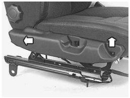
Pull the front edge of the panel upwards. Pull the panel backwards.
