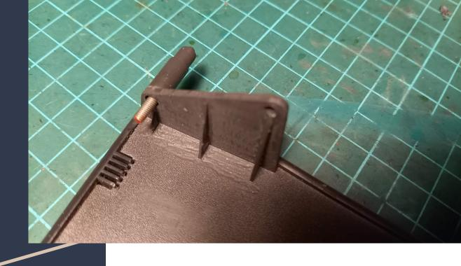
Then I made the surface rough for efficient sticking of glue.
