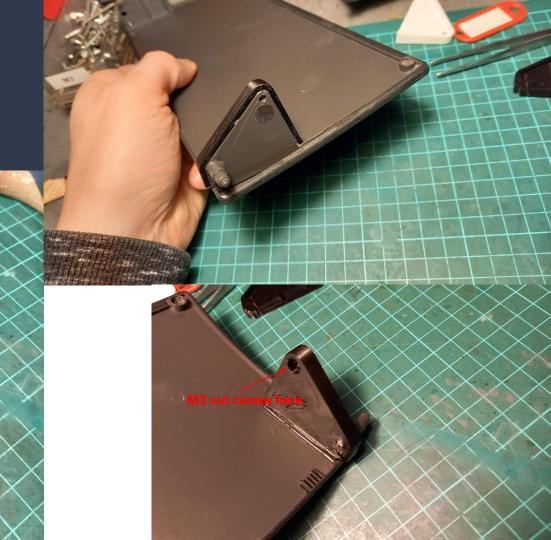
Two new shafts need to be manufactured. Raw material is an M4 hex socket screw partially threaded.
