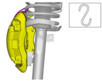
Warning! Make sure that no load is placed on the brake hose.
