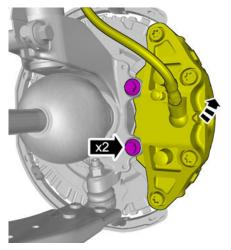
Warning! Make sure that no load is placed on the brake hose.
