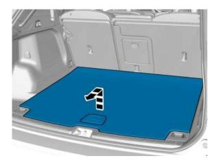
10. Use a small flat blade screwdriver to prise open and remove the recessed hard plastic cover on the cargo fixing point. Note that there is a small horizontal slot at the top of the recessed cover that allows the blade of the screwdriver to prise off the cover.
