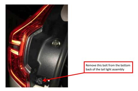
36. Loosen the black plastic impact absorber that sits below the tail light assembly and behind the wheel arch. It is held in place by 3 bolts. Remove the three bolts using an 8 mm socket.
