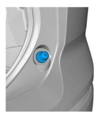
21. Remove all the Torx T25 headed screws from the underside of the bumper. There could be 4, 5 or 6 screws depending on the model variant.
