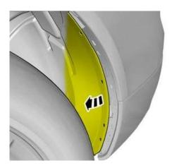
24. Remove the Torx T25 headed screw that fixes the bumper to the panel above it from the left side wheel arch.
