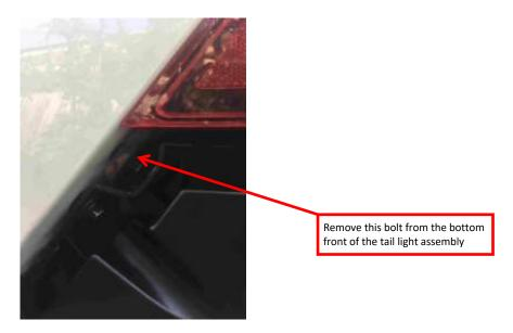
38. Partially pull out the tail light assembly and undo the electrical cable connector by pressing down on the release tab and pulling the connector away from the tail light assembly.
