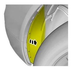
27. Remove the Torx T25 headed screw that fixes the bumper to the panel above it from the right side wheel arch.
