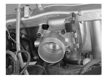
Disconnect the connector for the electronic throttle module.
