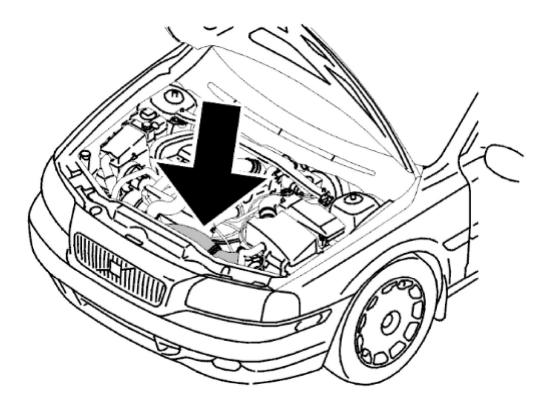
Install the charge air pipe between the electronic throttle module (ETM) and the charge air cooler (CAC).
