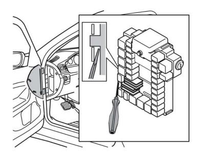
screwdriver so that the bracket opens out. At the same time, pull the relay box out of the bracket towards the underside of the dashboard. Lift the relay box off the bracket. Pull the relay box downward under the dashboard.
