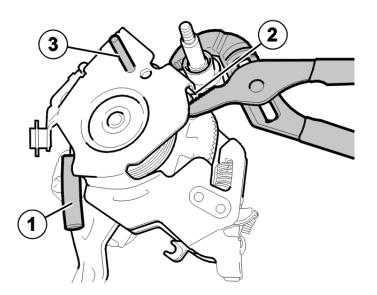
diameter of **5 mm** on the end of the friction spring (1). Open the friction spring so that the primary cable runs freely. Use a pipe wrench to push back the primary cable mounting (2). Insert a **6.5 mm** locking pin into the hole in the pedal (3) (it must pass through the bracket, cable pulley, pedal and the other bracket).
